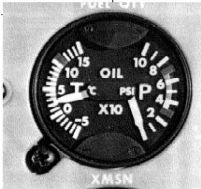
Figure 8-9 Transmission Oil Pressure/Temperature
